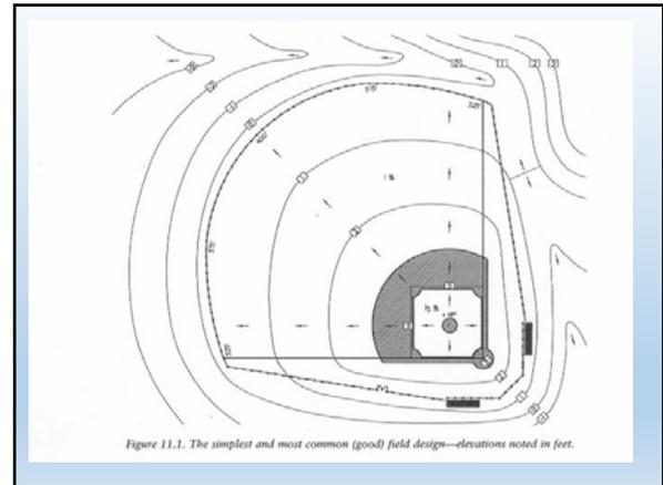
Figure 11.1. The simplest and most common (good) field design—elevations noted in feet.
