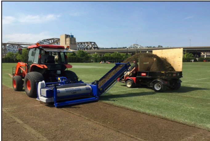
Fraze mowing Cincinnati Bengals practice facility – Photo courtesy of Darian Daily
