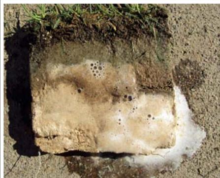
Calcareous soil effervescing when a drop of acid is placed on it as the carbonate ( $\text{CO}_3^{2-}$ ) converts to  $\text{CO}_2$  gas.
