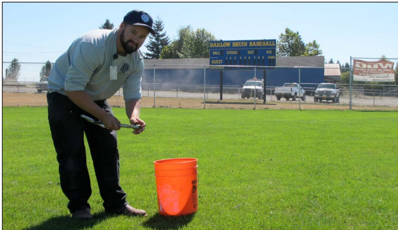
Figure 4: Collect 10 to 15 soil samples to a 4 inch depth using a soil probe, remove the thatch before placing the individual samples into a plastic bucket, and then mix the samples together for a composite sample.
