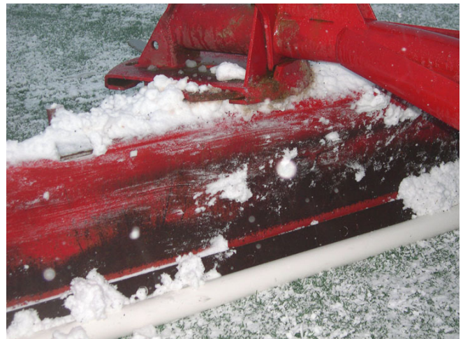
Figure 8. Attaching a split piece of 2-inch-diameter PVC pipe to the blade of this snowplow prevents the rubber infill material from being inadvertently removed from the artificial field when pushing snow. (Photo courtesy of Jason Bowers.)
