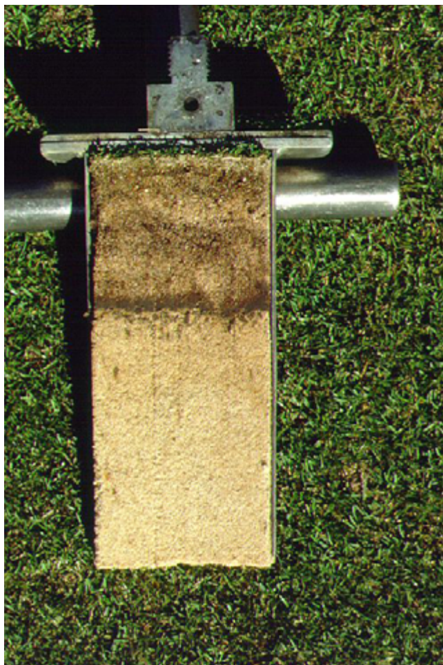
On golf greens especially, reducing or removing accumulated surface organic matter (thatch) is crucial under recycled water irrigation. Thatch and mat layers stop the flow of water through the soil and impede leaching of salts.
