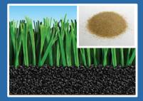
**Note:** No durability, performance, or safety issue Between <u>ambient</u> ground rubber and <u>cryogenic</u> rubber
