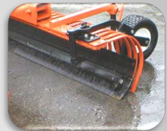
Modified manure spreaders with conveyor belts and brushes mounted on the back
