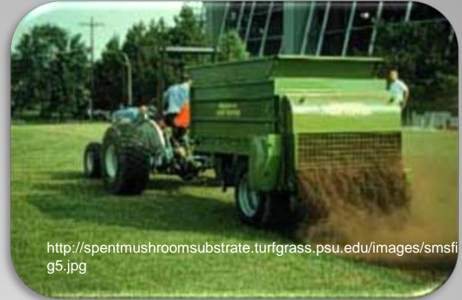
Modified manure spreaders with conveyor belts and brushes mounted on the back
