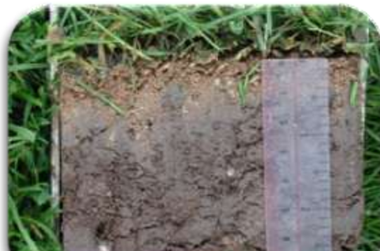
Sand topdressing, four applications (½” depth), applied over a 5-week period, Hancock Turfgrass Research Center, East Lansing, Michigan, July 27, 2008.
